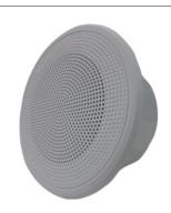
HN-D32N Noise Detector is designed to collect ambient noise samples and transmit the noise signal to the control system. The system can calculate the noise sound press level and adjust the output volume. It is intended for use in areas such as metro station, airport, shopping mall, where noise level varies constantly and sound clarity is of utmost importance.
